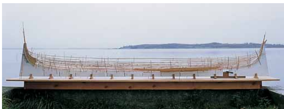
Fig. 41. Skuldelev 2. The working-model completed.
