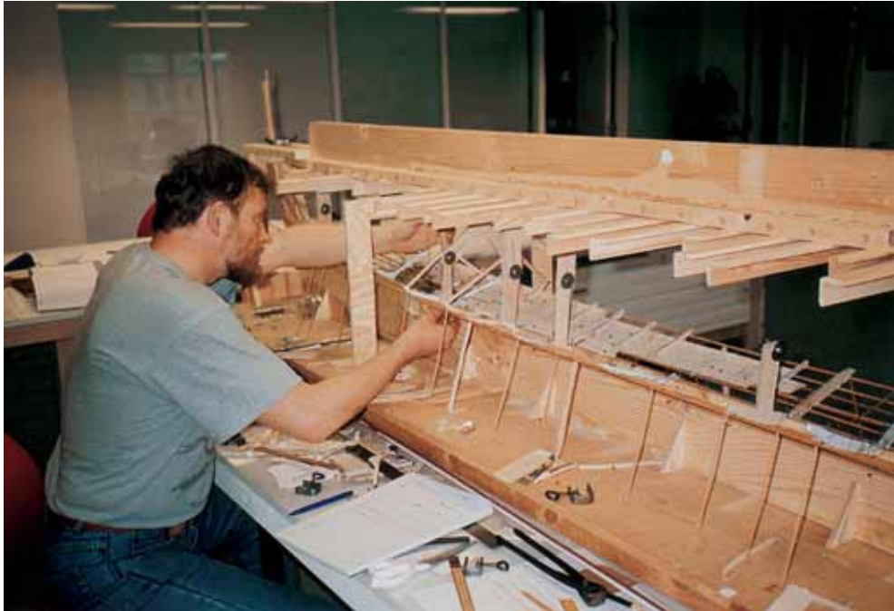
Fig. 39. Skuldelev 2. Working-model at scale 1:10 under construction.
