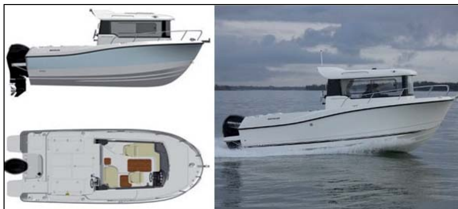
Figur 4: Orbicons surveyfartøj Sephia . Quicksilver Pilothouse 675.
