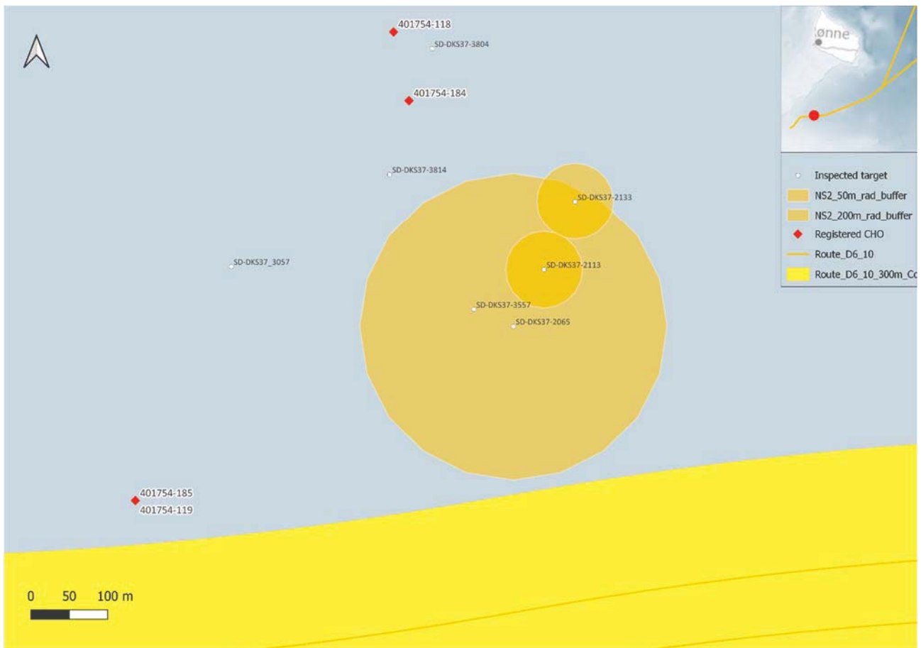
Figure 3. Map showing the different targets covered by the recommended exclusion zone of SD-DKS37-2065. Base map: Styrelsen for Dataforsyning og Effektivisering (Skærmkort, dæmpet, WMS-service). Bathymetry: EMODnet Bathymetry Consortium (2020): EMODnet Digital B.
